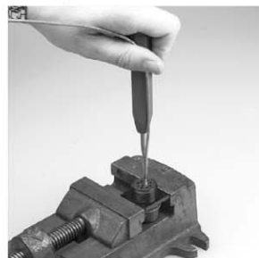
7. Use insertion tool to fully push contact into the receptacle insert.
