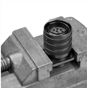
9. Place coupling ring then spring over plug shell before contact insertion.
