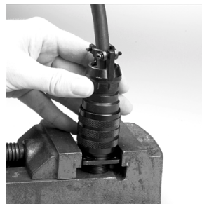
15. Ensure cable clamp is full threaded onto cable adapter.
