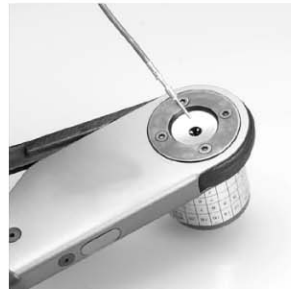
2. Fully seat contact in crimping tool.
