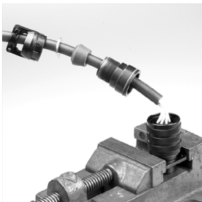
13. Plug with all contacts inserted, check that all contacts are fully seated.
