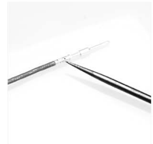
4. Inspect crimp for wire visibility through inspection hole.
