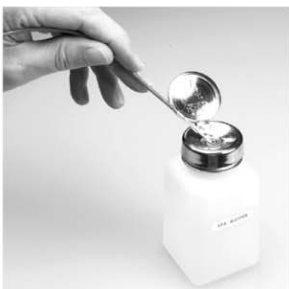
5. Use alcohol as a lubricant on contacts before insertion.
