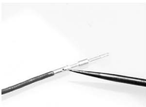
1. Insert stripped wire into contact pocket until it is visible through inspection hole.
